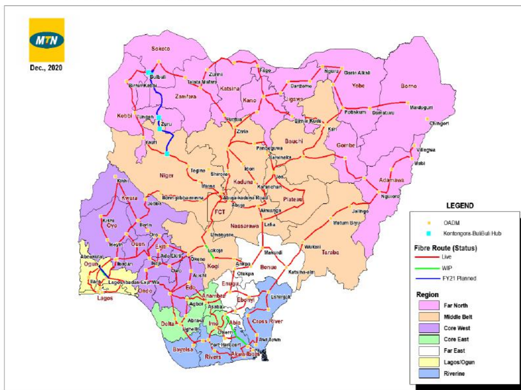
MTNN FIBRE BACKBONE NETWORK (PROJECT BLAZE)
